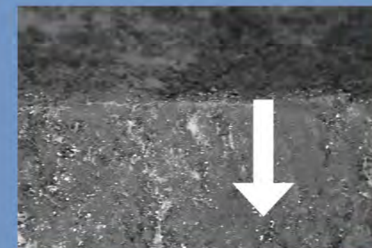
PFA penetrates deep inside pores and it melts inside graphite
