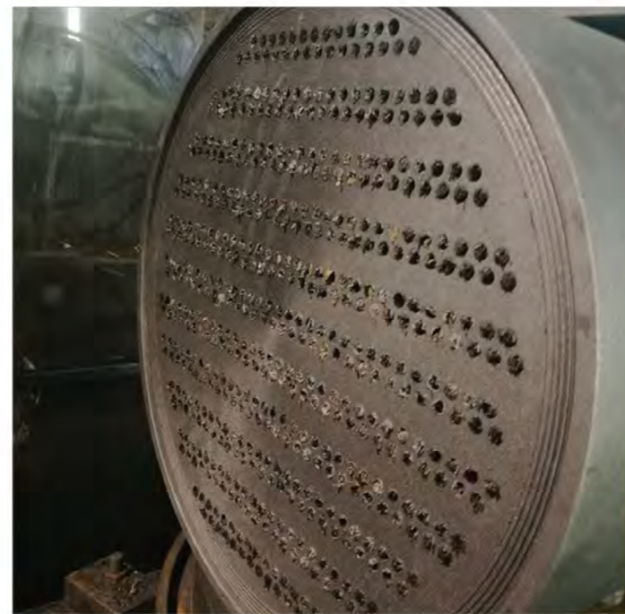
Round block after PFA impregnation (before cleaning)
